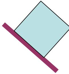
2. If the frictional force is assumed to be independent of velocity show that the effective acceleration of a block on a plane inclined at an angle  $\theta$  to the horizontal with coefficient of friction  $\mu$  is  $g(\sin \theta - \mu \cos \theta)$ .
