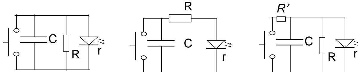
4. In the circuit below, how does the capacitor discharge when the dynamo stops?
